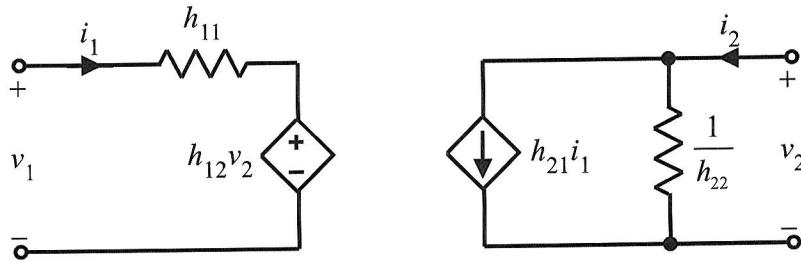
Hybrid parameters are useful for combining two two-port networks that are connected together in a **Series-Parallel** configuration. The hybrid parameters conveniently add together, as shown below:
